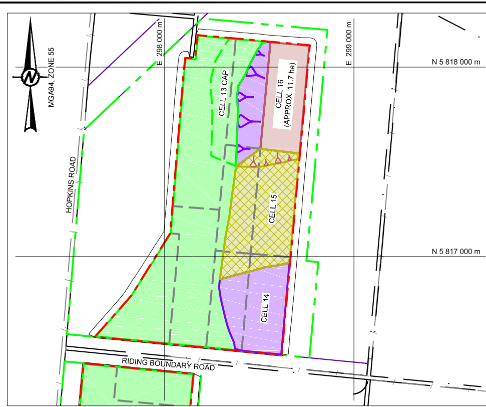
STEP 16 CELL CONSTRUCTION: CELL 16 BASE LINER WASTE FILLING: CELL 15 CAPPING: FINAL CAP CELL 13, INTERIM CAP CELL 14
