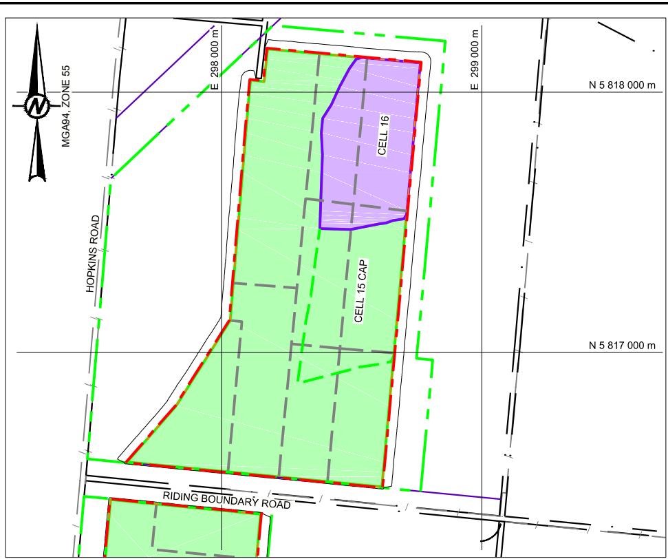
STEP 18 CAPPING: FINAL CAP CELL 15, INTERIM CAP CELL 16
