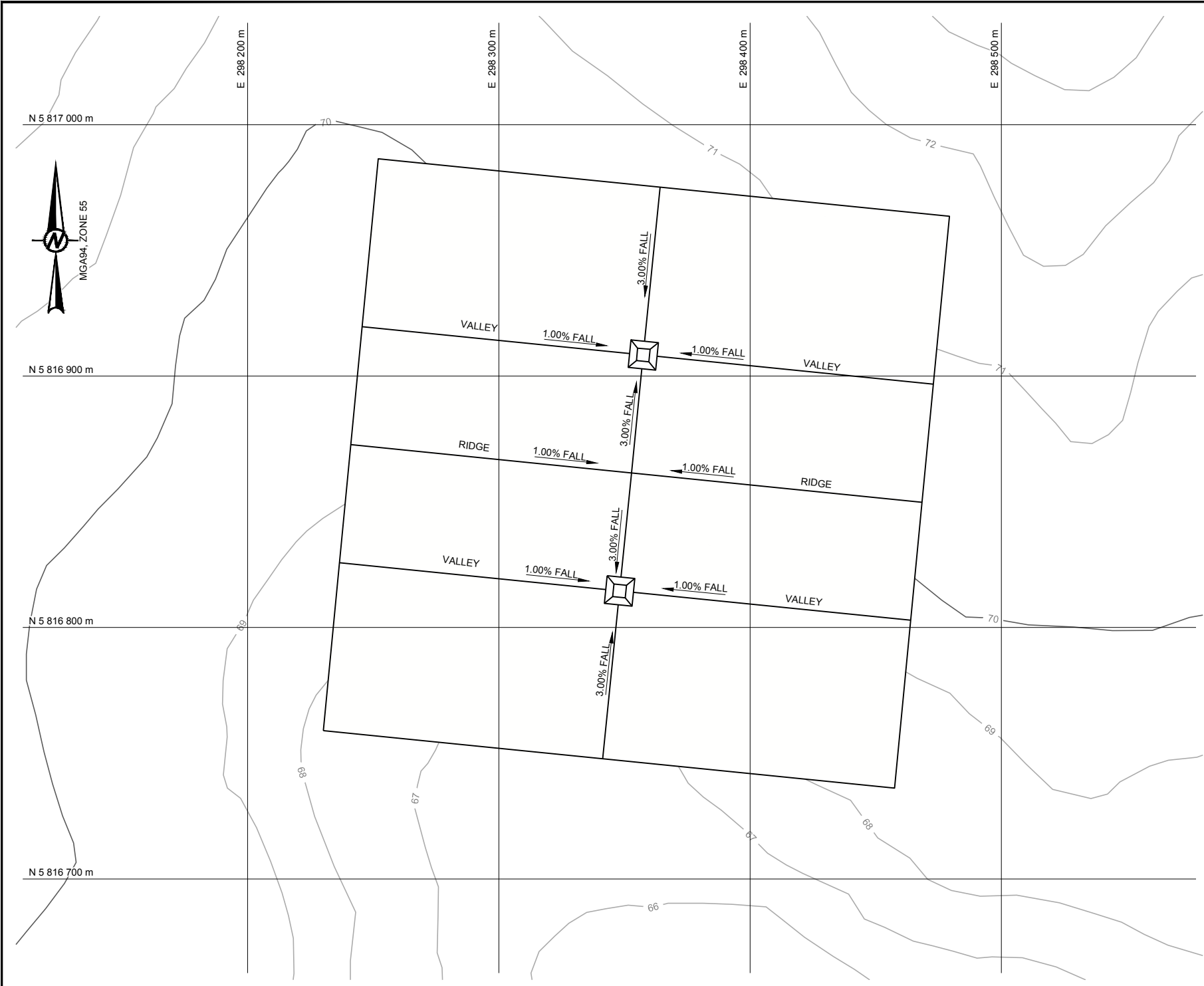
TYPICAL SUBGRADE FLOOR PLAN - INTERNAL SUMP SCALE 1:2,000
