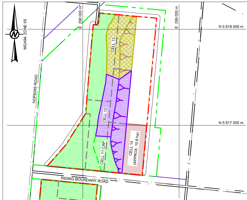
STEP 14 CELL CONSTRUCTION: CELL 14 BASE LINER WASTE FILLING: CELL 13 CAPPING: FINAL CAP CELL 11, INTERIM CAP CELL 12
