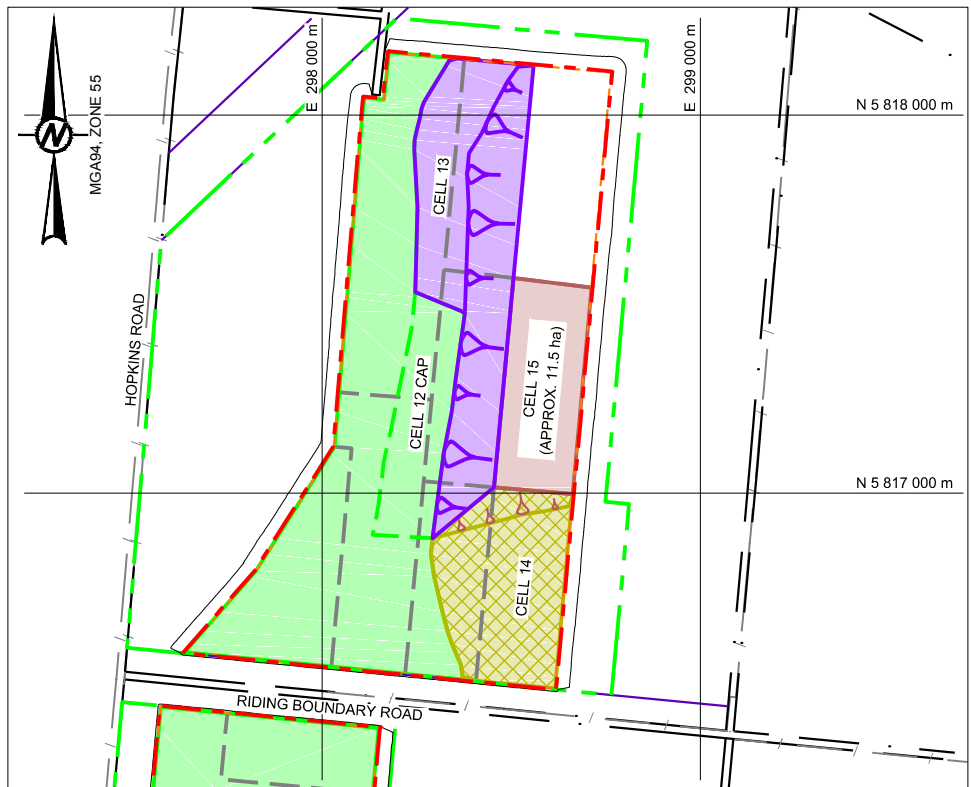
STEP 15 CELL CONSTRUCTION: CELL 15 BASE LINER WASTE FILLING: CELL 14 CAPPING: FINAL CAP CELL 12, INTERIM CAP CELL 13
