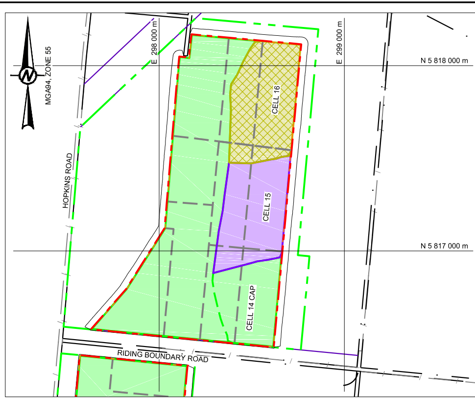
STEP 17 WASTE FILLING: CELL 16 CAPPING: FINAL CAP CELL 14, INTERIM CAP CELL 15
