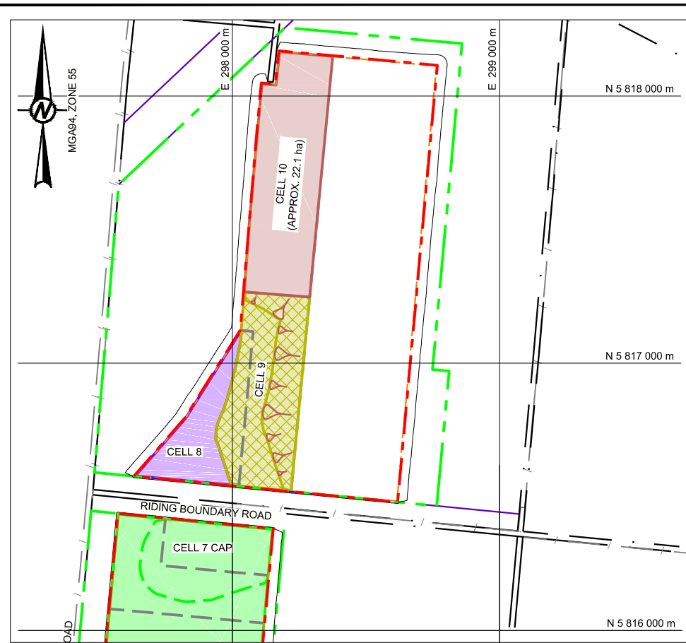
STEP 10 CELL CONSTRUCTION: CELL 10 BASE LINER WASTE FILLING: CELL 9 CAPPING: FINAL CAP CELL 7, INTERIM CAP CELL 8
