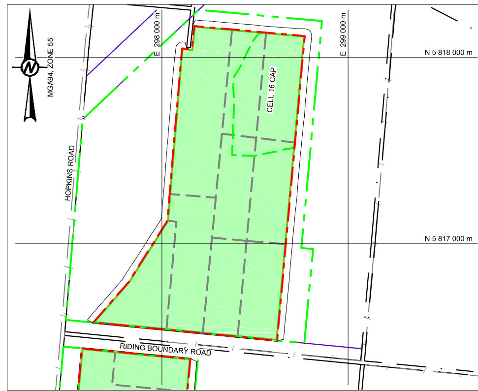
STEP 19 CAPPING: FINAL CAP CELL 16
