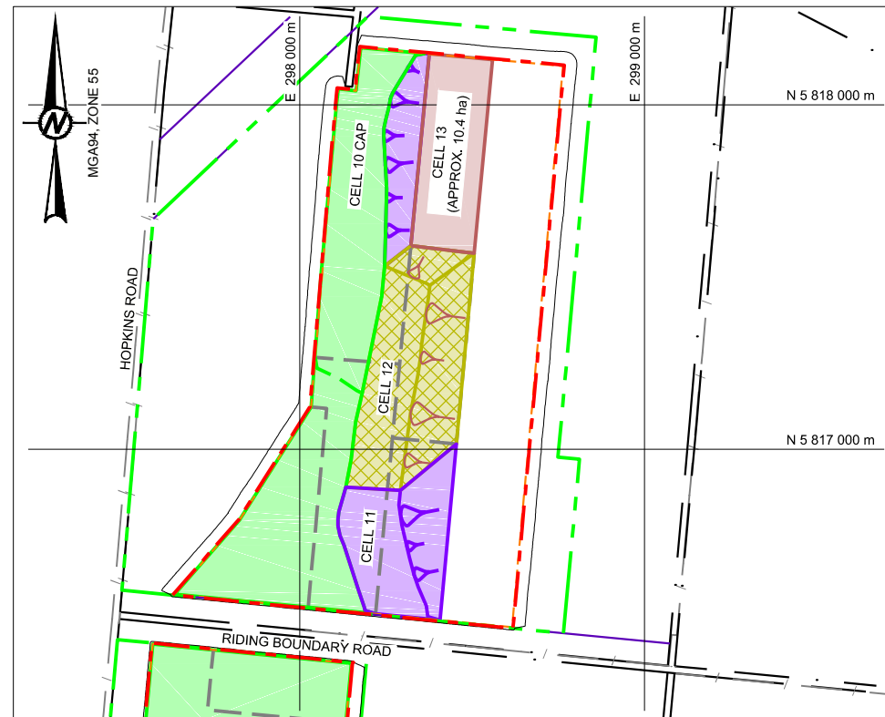
STEP 13 CELL CONSTRUCTION: CELL 13 BASE LINER WASTE FILLING: CELL 12 CAPPING: FINAL CAP CELL 10, INTERIM CAP CELL 11
